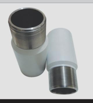
The blast joint is used to protect the tubing string against the "gas jet" abrasive effect when positioned in front of the perforations.
